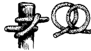
The clove hitch is used for making a line fast temporarily to a pile or bollard.
