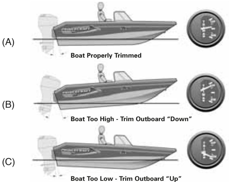
FIGURE 7-3 TRIMMING THE BOAT OUTDRIVE
