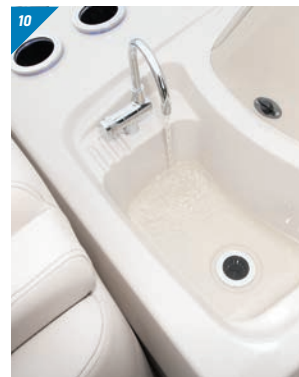
1 Tilt steering wheel 2 Pop-up privacy enclosure 3 Premium High Power/Sub Audio System 4 Multifunction Simrad® Go9 touch screen 5 SmartCraft™ instrumentation 6-7 Chemical head 8 Stainless steel waterski tow bar 9 Battery switch 10 Console galley conversion (sink, faucet, electric pump, and water tank) 11 Active Trim (automatic trim setting) 12 SeaStar® hydraulic steering system with tilt wheel
