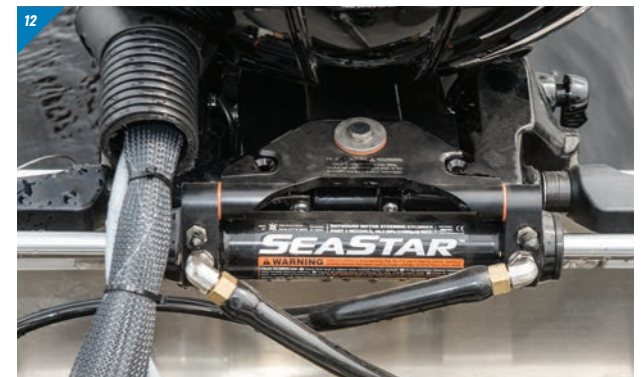
1 Tilt steering wheel 2 Pop-up privacy enclosure 3 Premium High Power/Sub Audio System 4 Multifunction Simrad® Go9 touch screen 5 SmartCraft™ instrumentation 6-7 Chemical head 8 Stainless steel waterski tow bar 9 Battery switch 10 Console galley conversion (sink, faucet, electric pump, and water tank) 11 Active Trim (automatic trim setting) 12 SeaStar® hydraulic steering system with tilt wheel
