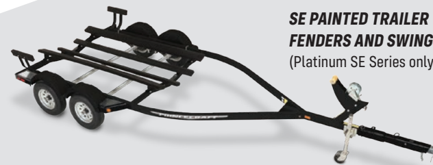
SE GALVANIZED STEEL TRAILER WITH STEEL FENDERS AND SWING TONGUE (Platinum SE Series only)
