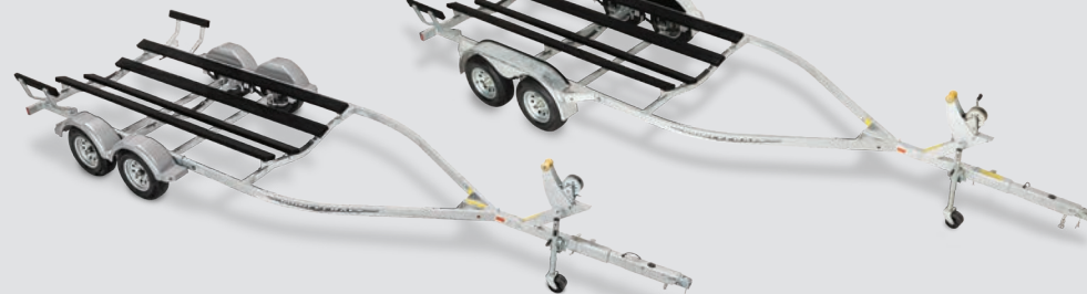
GALVANIZED STEEL TRAILER WITH SWING TONGUE
