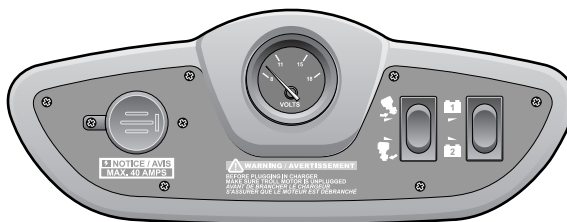
FIGURE 4-4 12-24 VOLT BOW TROLLING PANEL
