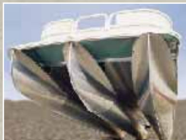
Princecraft P3 package (Pontoon Performance Package) Our new P3 package adds a center log and aluminum under body splash panel. The extra log gives the boat more capacity an added performance capability, while the under body splash panel tames wave action for smoother running at higher speeds. (Available on Versailles Series)
