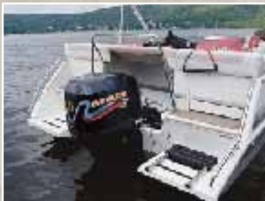
Waterski Tow Bar This stainless steel waterski tow bar is welded and bolted to the boat's main structure for maximum strength and durability. It is specifically designed to fit all Princecraft deck boat models and provide maximum towing ability.
